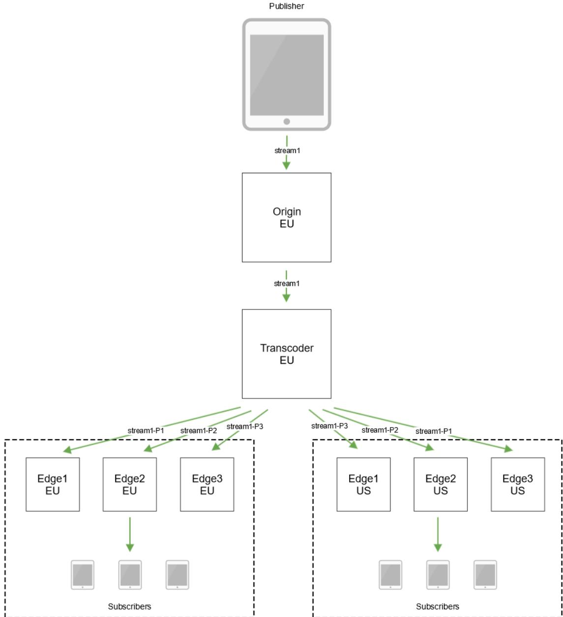
In this case, the stream is transcoded one time for all location groups, but as many streams will be broadcast to each group as requested by Edges for playback. This increases intergroup channels load.
