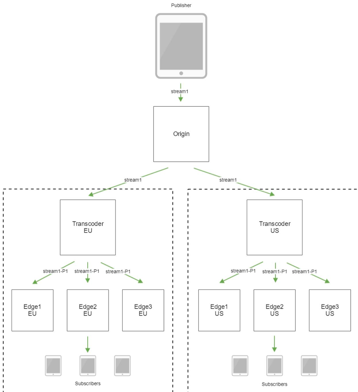
In this case, only one stream will be broadcast from Origin to each group, this decreases intergroup channels load, but stream will be transcoded in every group independently.
