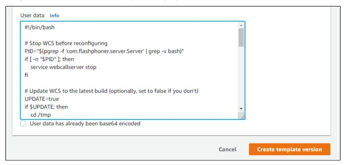
The setup script example to update WCS to latest build and to configure CDN Edge server for WebRTC playback
