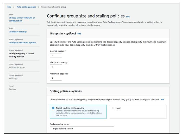
2.10. Select scaling policy by CPU utilization, set target value and instance warming time
