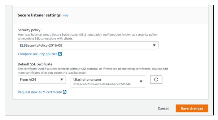
Load balancer listener parameters are changed and will be applied immediately
