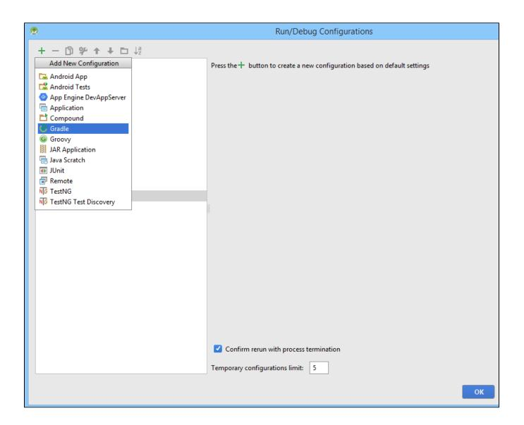
5. To configure the run, specify the build gradle file, the name of the build and set the purpose to: build
