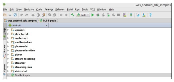
The building result is .apk files located in the corresponding folders: 2players/build, click-to-call/build, and so on. The Android SDK file is located in the following path in the project: libs/wcs-android-sdk-1.0.1.2.aar
