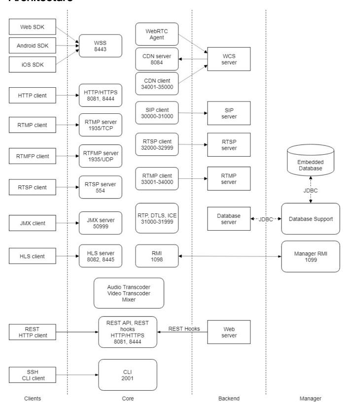
WCS works under Linux x86\_64 operating system. The network architecture of WCS is shown on the above picture and has two main modules:
