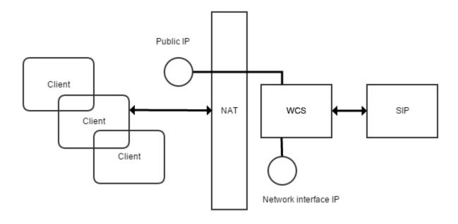
When the WCS server is to deployed behind NAT, you need to discover two IP addresses.
