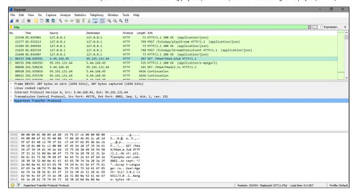
To track playback of a given stream, use the "Follow HTTP stream" function of Wireshark:
