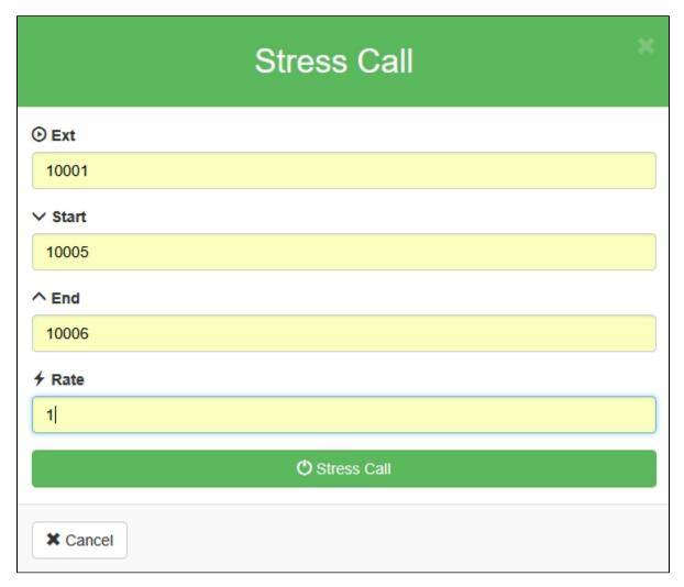
7. Press 'Stress Call' button. The test begins. In 'Show' dropdown select 'TESTS' and press 'Apply'. The information about test passing will be displayed on the page:
