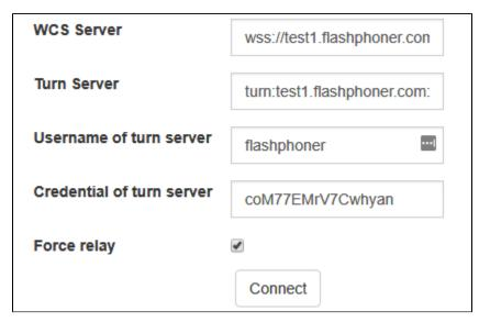
$4.\ Press{\tt Connect}, enter stream \ name{\tt test} and \ press{\tt Publish}. \ Stream \ publishing \ starts \ through \ internal \ TURN \ server.$
