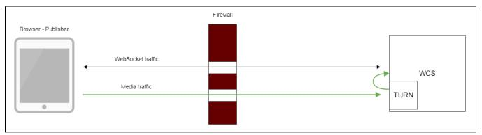
Client browser establishes TCP connection to internal TURN server port (3478 by default), then internal TURN server connects to local WCS interface through UDP ports from specified range (36001-37000 by default). Thus, for client media traffic flows through TCP tunnel, and for WCS server nothing is changed, traffic flows via UDP ports.
