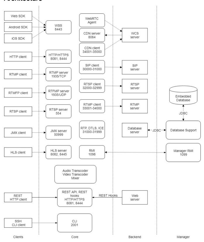
WCS works under Linux x86\_64 operating system. The network architecture of WCS is shown on the above picture and has one main module:
