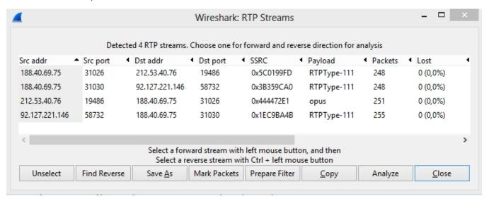
In this specific case RTP traffic is represented by streams with SSRC 0x5C and 0x44.
