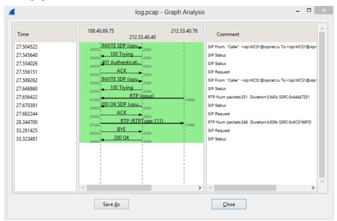
From the analysis of the SIP call we can see that WCS receives and sends RTP audio streams with audio data encoded by Opus.
