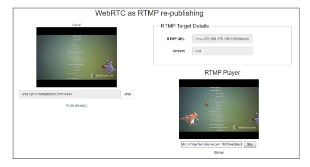
In RTMP player window set URL and name of the channel output stream created at step 3
