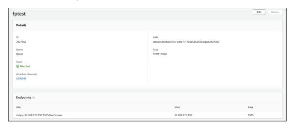
3. AWS MediaLive configuration: Create channel with Output group: RTMP
