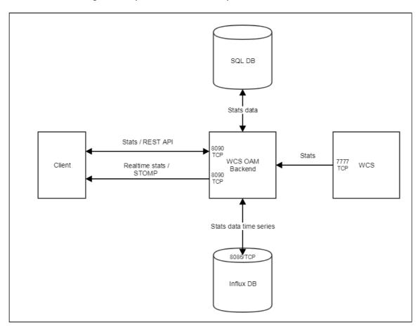
Backend server allows to monitor a couple of WCS servers simultaneously.
